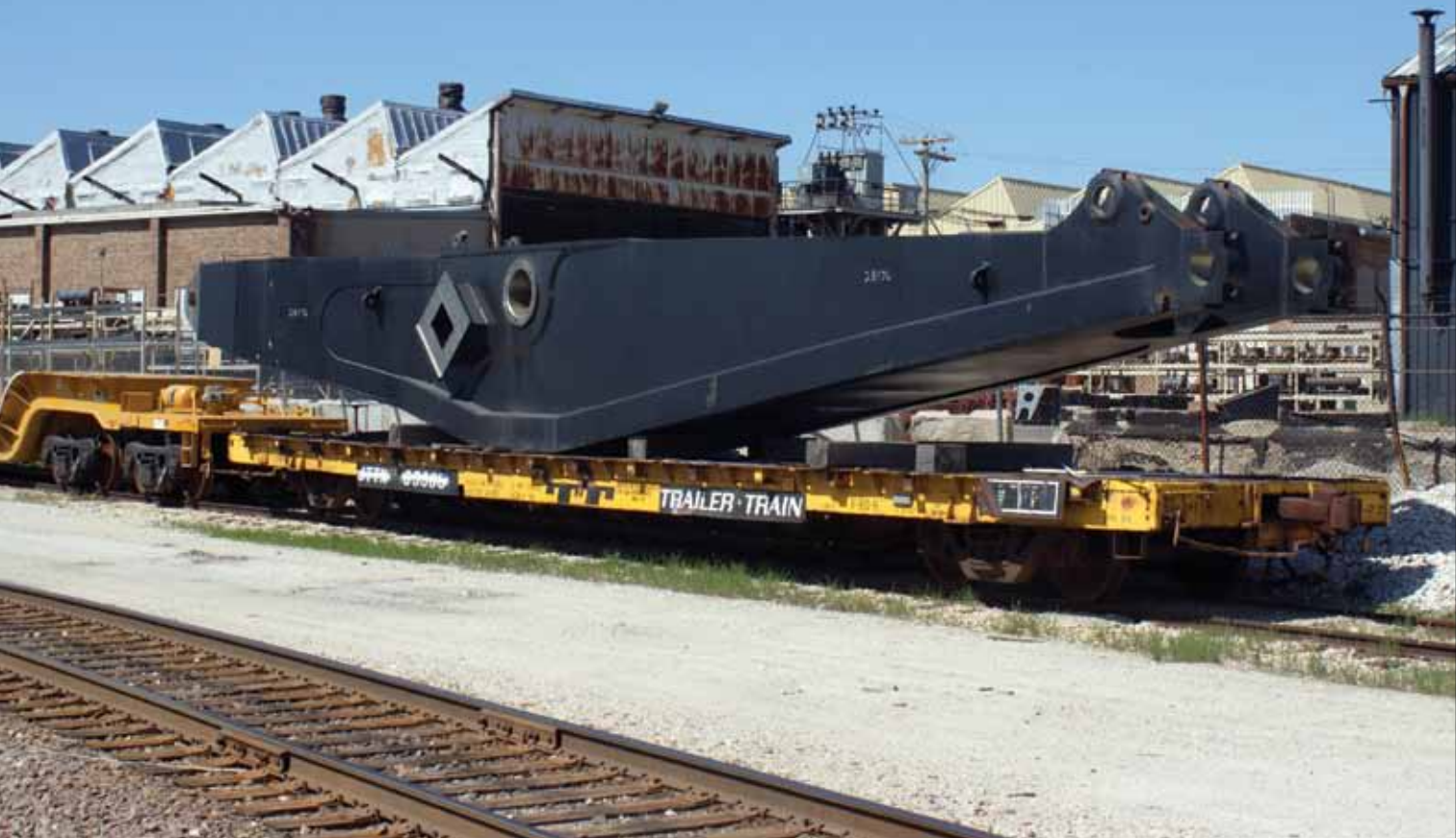
P&H makes its equipment in pieces and ships it to mine sites, where another affiliate of its parent company, Joy Global, performs the assembly. The boom eye that the company is currently targeting for casting conversion is at the left end of this boom.
