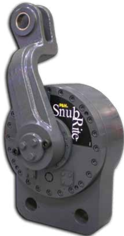
This snubber arm casting replaced a steel fabrication and keeps the 25,000-lb. dipper door on P&H's electric mining shovels from opening and closing too fast.
