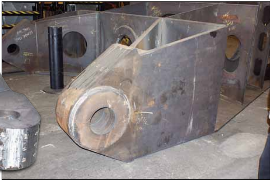
This fabricated boom eye (shown before assembly in the inset) is P&H's current target for conversion to casting. To produce the fabrication, P&H must process multiple steel plates and weld them together.
